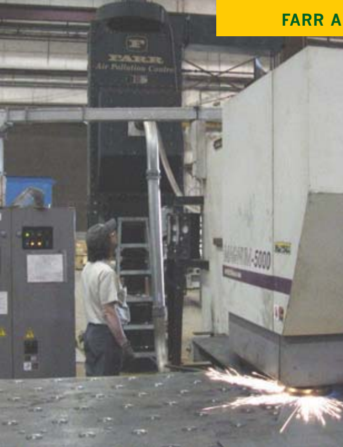
CNC Plasma Cutting with GS2 Dust Collector
